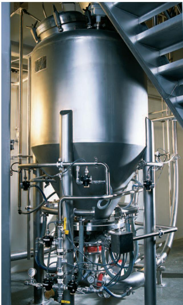
**A pneumatic blender requires little or no cleaning in most applications because it has few moving parts in contact with the material.**
