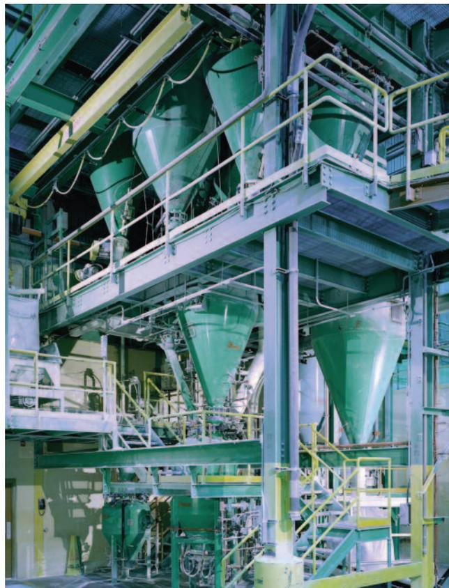
**Installing a pneumatic blender in a hopper, as shown here (bottom center), minimizes the overall equipment footprint required for a mixing process.**
