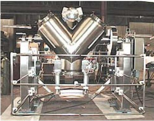
There are three commonly recognized shapes of tumble blenders, the V-shape, double cone and slant cone (Gemco trademark). There is also a significant distinction between symmetrical and asymmetrical designs within the three shapes.
