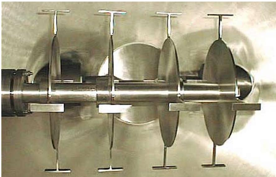
*(Photo above is a large, 4-disc internal agitator bar used for delumping and breaking up agglomerates of minor ingredients and extending minor ingredients.)*
