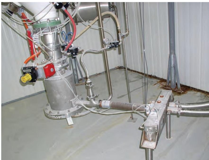
***The granular salt discharges from the Mini-Jet at about 500 fpm and moves through a diverter valve, which directs it into the proper conveying line.***
